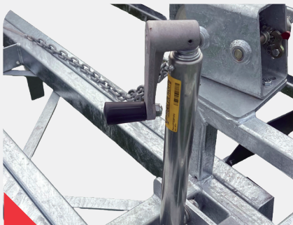
Front to back and sideways levelling system.
